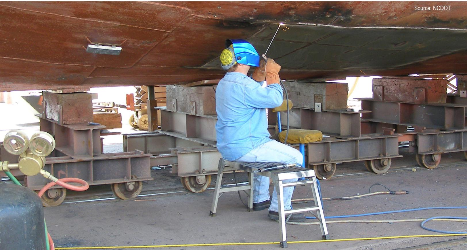
Image Caption: A boat welder works on a steel hull plate for an NCDOT ferry vessel.
